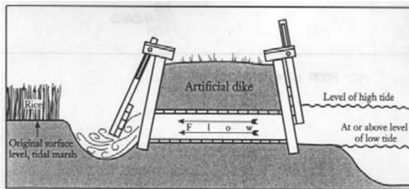
Cross Section of Embankment Showing Operation of Trunk and Flood Gates
